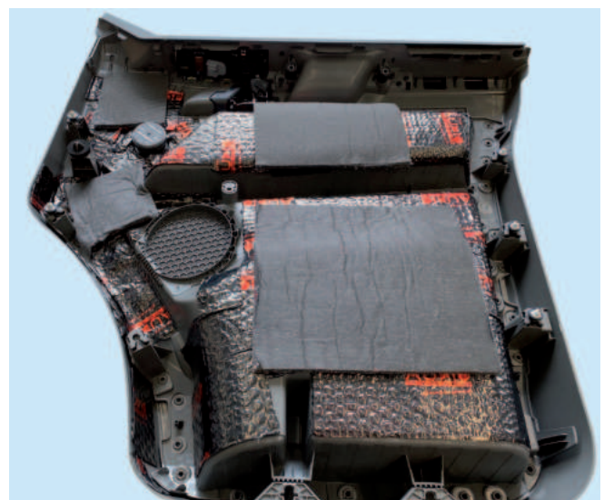
Second insulation layer with insulating fleece mats
