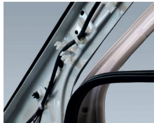
1a.6 Carefully lever out the A-pillars with the plastic wedge and remove them from the vehicle in twos.
