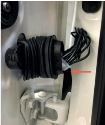
4b.1. lead the subwoofer cable through the rubber sleeves into the vehicle door and behind the behind the door panel to the pre-drilled to the subwoofer behind the door trim.
