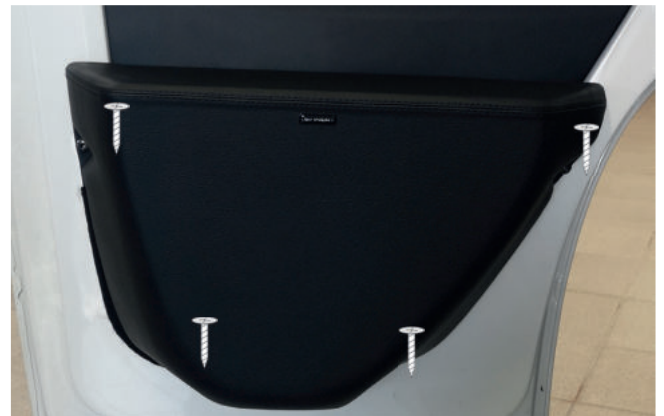
4a.17. Connect the subwoofer and mount it with the factory screws. mount the screws of the card compartment; place the supplied 4 rubber rings between the back of the subwoofer and the door trim.
