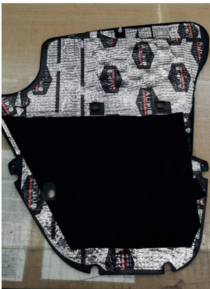
4a.9 Recommendation: Insulate door trim with Alubutyl and acoustic foam mat. (Only with insulation package (optional accessory)).
