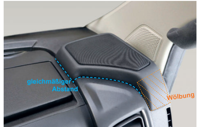
1b.2. JEHNERT mid-range module without loudspeakers on the dashboard. Align the dashboard: Place the curvature of the module against the curvature of the dashboard and ensure that there is an even distance between them.
