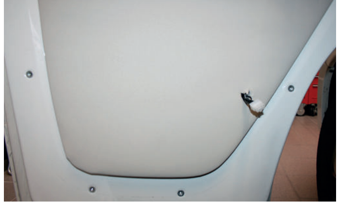
4b.2. grommet for the subwoofer cable after installation seal against moisture
