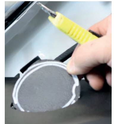
1a.4. heat the marked cutout well with a hot-air dryer and cut out with a sharp cutter knife.
