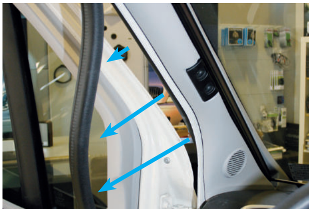
1a.5 Loosen the rubber door seal in the A-pillar area.
