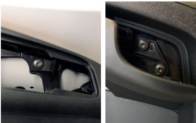
4a.16. Tighten the screws under the power window control panel and the door opener and clip on the covers.
