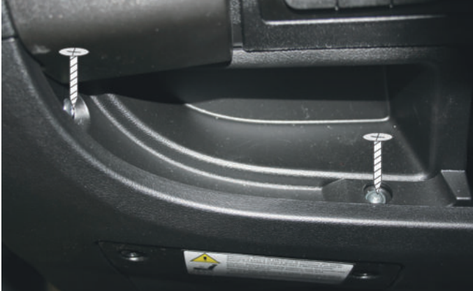
4c.1. Loosen 2 screws on the left below the steering wheel.
