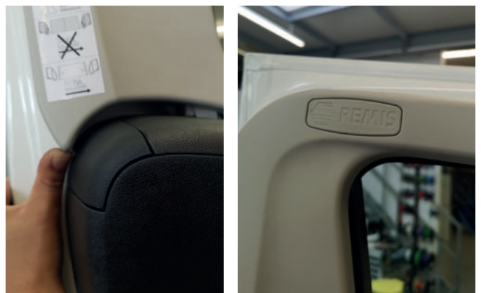
Tighten the upper left screw of the door trim again. Cover and screw „REMIS“ roller blind „REMIS“ roller blind screw tight again
