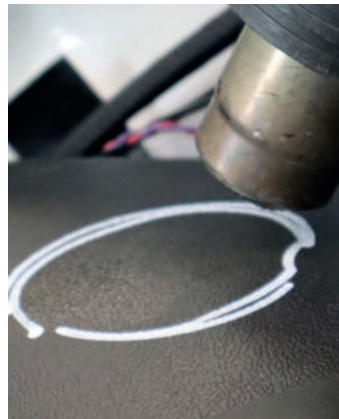
1a.4. heat the marked cutout well with a hot-air dryer and cut out with a sharp cutter knife.
