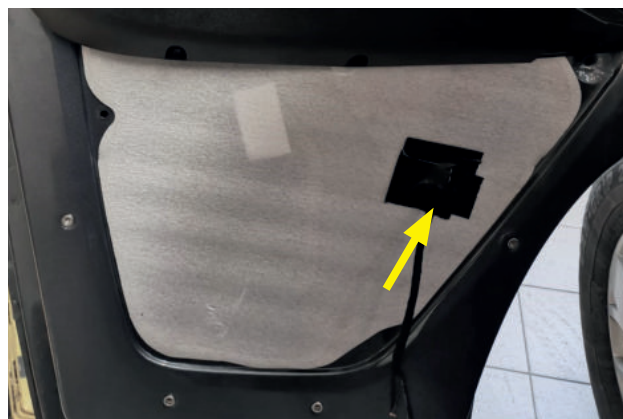
4a.11. Slightly cut the foam in the area of the subwoofer cable hole slightly, feed the subwoofer cable through and tape it and seal tightly with adhesive tape.
