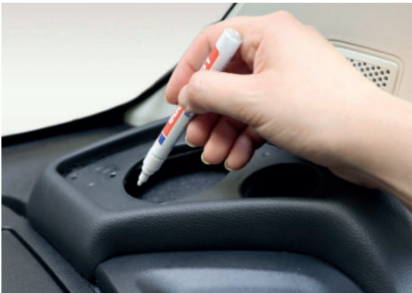
1a.3 Mark the speaker cutout on the dashboard (white marker).
