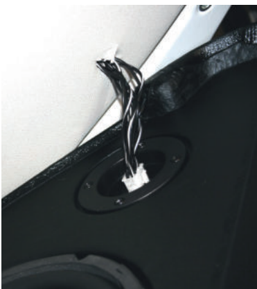
4b.5. connect the connection cable and fix the subwoofer with the screws and rubber rings supplied with the subwoofer. to the door panel using the screws and rubber rings supplied
