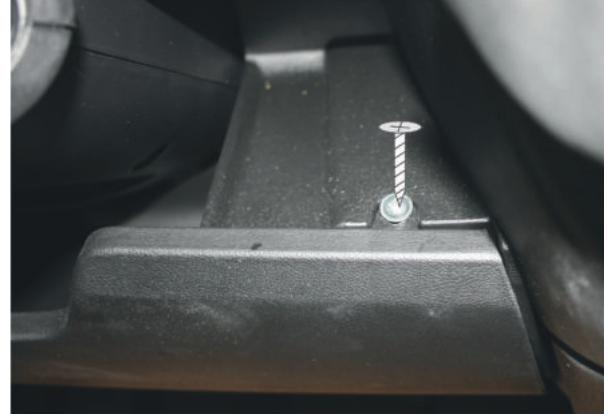
4c.2. Loosen 1 screw on the right underneath the steering wheel and remove cover.
