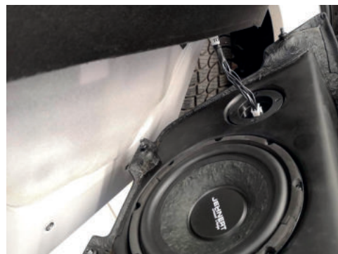
Refit door panel and leave cable hanging approx. 20cm
