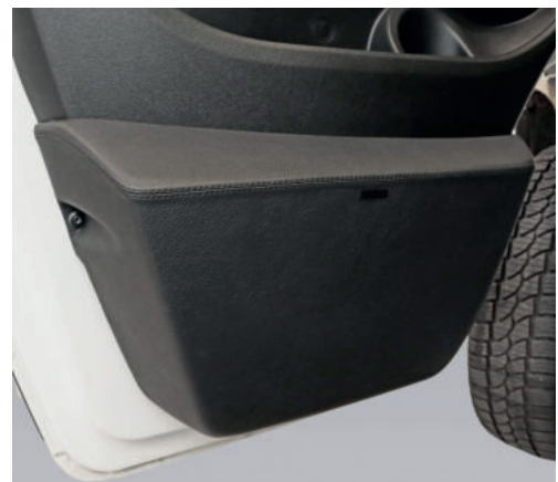
Refit door panel and leave cable hanging approx. 20cm
