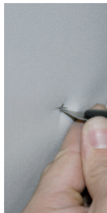
4b.2. grommet for the subwoofer cable after installation seal against moisture
