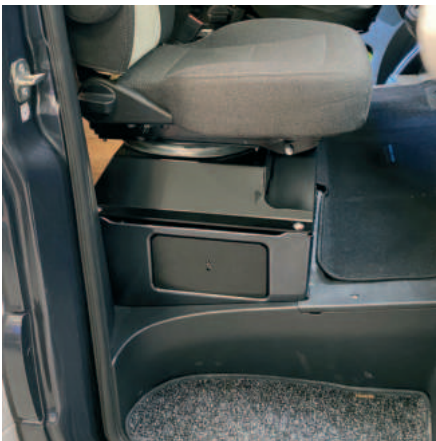
Safe'n'Sub in the Sprinter, mounted under the passenger seat
