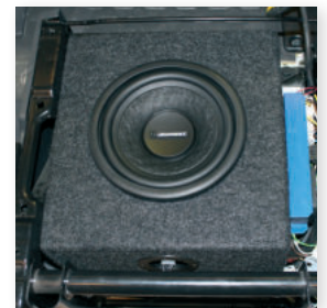
»17014« Subwoofer under the seat in the Fiat Ducato (seat console under the passenger seat)
