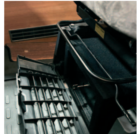
Safe'n'Sub mounted under the passenger seat (Fiat Ducato)
