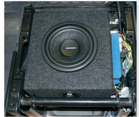
»17014« Subwoofer under the seat in Fiat Ducato (seat console under passenger seat)
