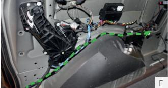
• Run the cable up to the wheel housing and along above the wheel housing to the subwoofer connection point.
