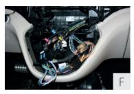
• Pull ISO cable through radio slot, center console to under passenger seat
