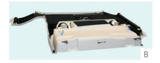
• Insulate the back of the roof lining with insulation fleece
