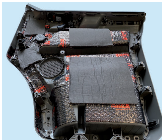
Second insulation layer with insulation fleece mats
