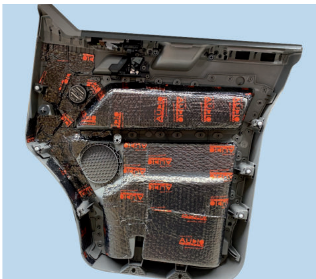
First insulation layer with alubutyl mats
