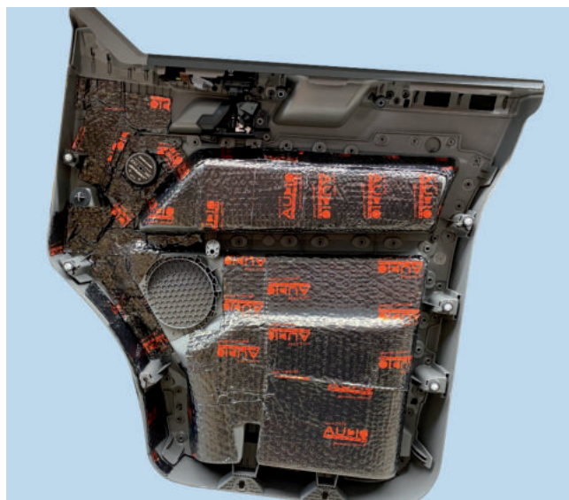
First insulation layer with alubutyl mats
