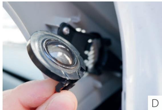
**C:** Carefully remove A-pillar trim, place on dashboard (->protect surface with adhesive tape if necessary) and unclip and unplug existing original tweeter
