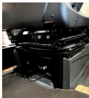
Subwoofer »17011« installed under the driver's seat
