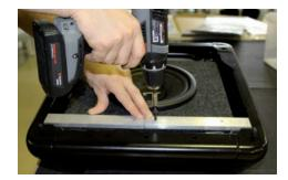
Attach mounting bracket and secure with 4.8 x 22 to secure.
