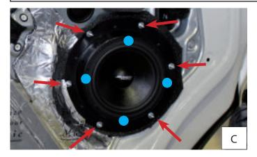
3.1 Fasten the mounting ring with 6x M5 x 30 screws, 5mm washers and M5 polystop nuts each (Fig. C). Then fasten the loudspeaker to the mounting ring with 4x 3.9 x 16 raised countersunk head screws each and connect the original loudspeaker connector with the JEHNERT loudspeaker connector and the JEHNERT loudspeaker.
