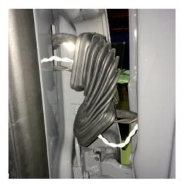
2.5. lead the woofer cable to the woofer installation location through the rubber grommet to the vehicle door.
