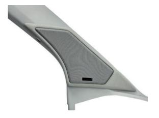
6.7 Reassemble the A-pillar trim and Attach cover panel
