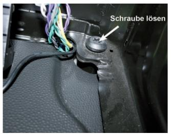
7.3 Loosen the screw on the seat console and feed the ISO cable underneath.
