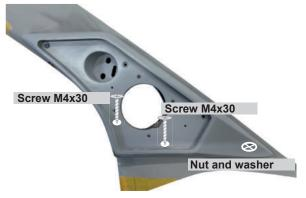
6.4 Align the module on the A-pillar and mount it with the supplied screws as shown in the illustration. Insert the screws through the holes previously drilled in the A-pillar -->> Screw the screws with washer and self-locking nut and tighten carefully! (Illustration for better representation without speakers)
