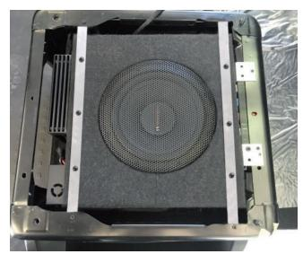
7.4 Mount the amplifier on the subwoofer and connect it with the "plug & play" cable, insert it into the seat console and screw it to the seat with strips on the frame of the seat console.
