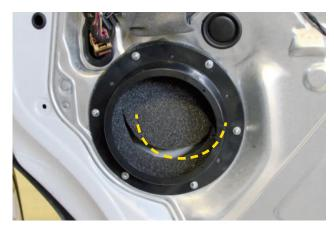
3.1. Cut the Rainstop mat to the size of the mounting ring. and make a circular cut in the lower area. Place the mounting ring with the Rainstop mat on the factory opening with the 6 screws supplied (M4 x 20 (M4 x 20 - hexagonal). At the front and rear, shim with 12 mm washers at the front and rear.
