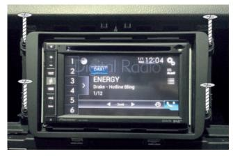
2.2 Remove the 4 Torx screws (TX20) underneath.
