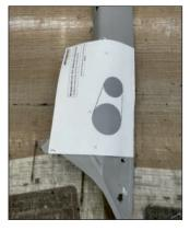
6.3 Place the enclosed template on the A-pillar, mark the speaker openings and cut them out with a jigsaw. **Caution:** do not cut away too much
