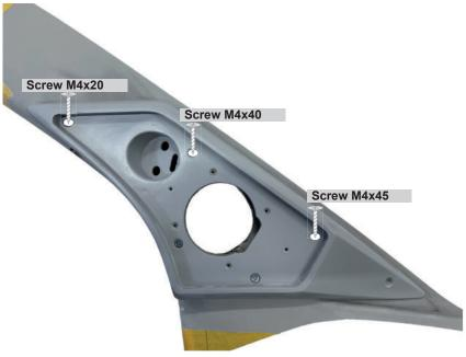
6.5 Use the remaining screws to fix the molded part to the A-pillar.
