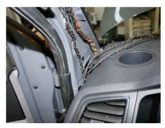
2.6 Route the mid-range and tweeter cables under the dashboard to the A-pillar.
