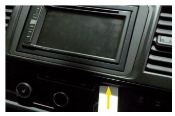
2.1 Use a plastic wedge to lever off the radio bezel (incl. ventilation nozzles). lever off with a plastic wedge.
