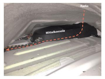
7.2. ISO cable from the radio, under the carpet and under the center console cover to the passenger seat console. lead.
