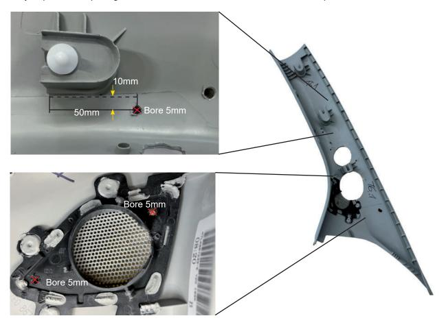
6.2 Drill holes (5mm Ø) on the back of the A-pillar for the screw anchored in the molded part. The drilling points are located on the reference point of the factory tweeter mounting.
