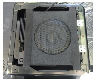
7.5. subwoofer ready mounted and strips covered with covered with felt fabric.
