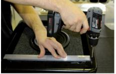
Pre-drill the screw holes for fastening to the Pre-drill the seat bracket (slightly countersink the drill hole).
