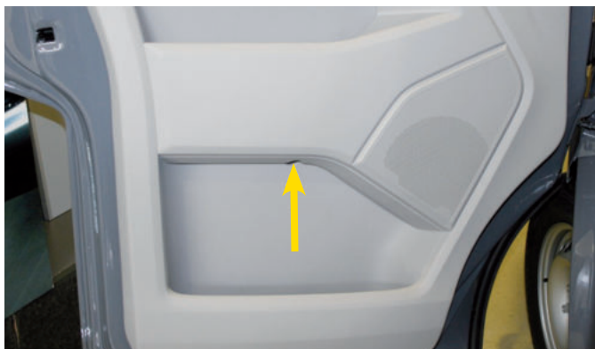
1.4. remove the screw in the middle of the door panel.
