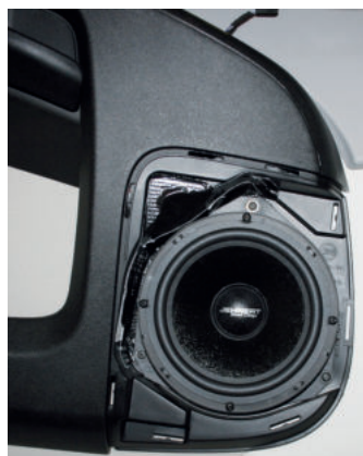
2a.4. mount the woofer adapter with the factory screws. Connect and mount JEHNERT woofer. Put on the loudspeaker cover.
