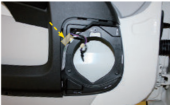
2a.3. run factory speaker cable between door panel and plastic trim behind the woofer opening (see fig. marked area).
