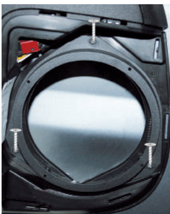
2a.4. mount the woofer adapter with the factory screws. Connect and mount JEHNERT woofer. Put on the loudspeaker cover.
