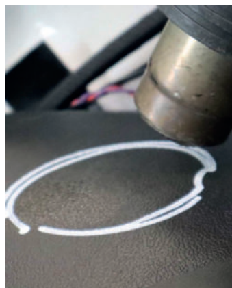
1.6 Heat the marked cutout well with a hot air dryer and cut out with a sharp cutter knife.
