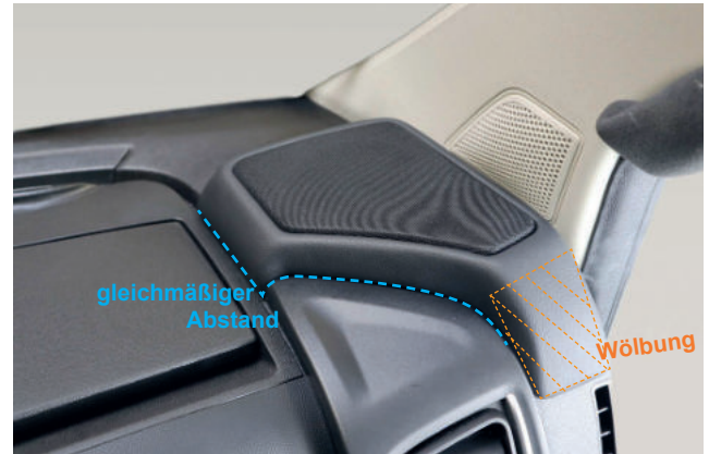
1.2 JEHNERT midrange module without loudspeakers on the dashboard. Align the dashboard: Place the curvature of the module against the curvature of the dashboard and ensure that there is an even distance between them.
