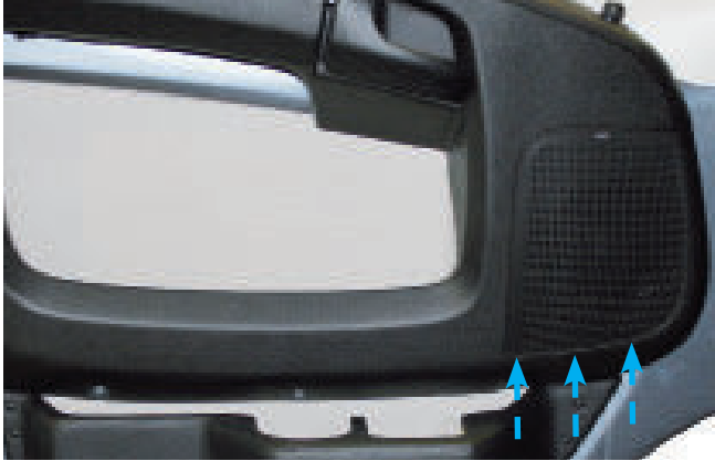
2a.1. lever out the loudspeaker cover in the vehicle door from below, starting from the bottom (with plastic wedge).
