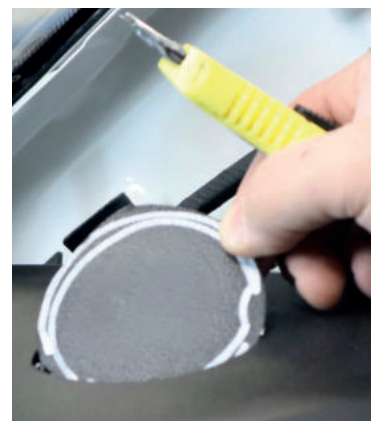
1.6 Heat the marked cutout well with a hot air dryer and cut out with a sharp cutter knife.
