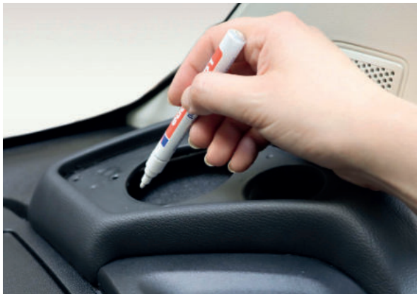
1.3 Mark the speaker cutout on the dashboard (white marker).
