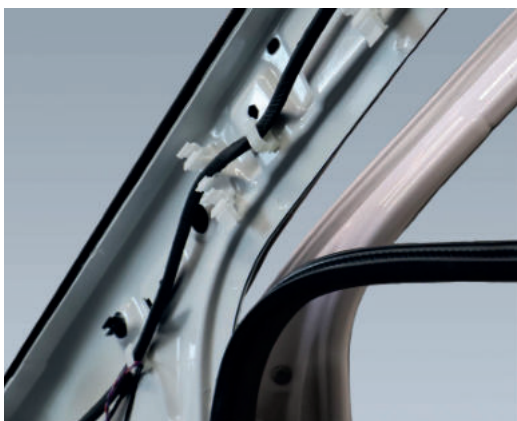
1.5 Carefully lever out the A-pillars with the plastic wedge and remove them from the vehicle in twos.
