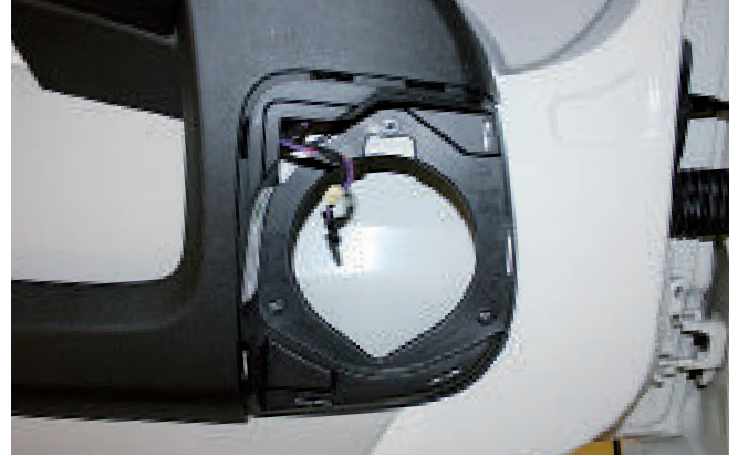
2a.2 Dismantle the factory loudspeaker and disconnect the connection cable. The factory screws are used for fastening the JEHNERT low-frequency adapter.
