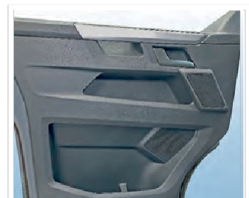
Midrange module in the door panel for models with blackout roller blind
