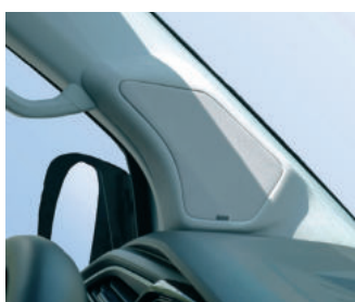
Mid-high module in the driver's side A-pillar
