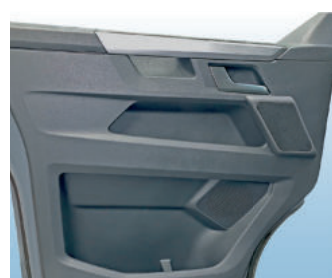
Mid-range module in the door panelling for models with blackout blind
