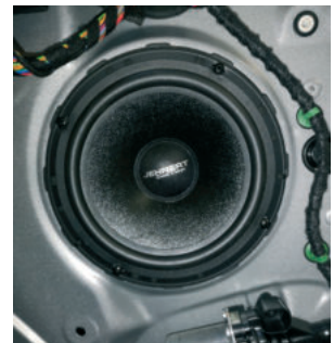
Woofers installed in factory mounting locations
